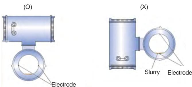
Electromagnetic flowmeter must work in full pipe conditions, that is to say, the flowmeter cannot work normally in partially filled pipe or empty pipe conditions.
