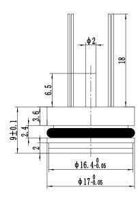
The suggested installation dimension is: $\Phi$ 17  $^{+0.05}_{+0.02}$ mm
